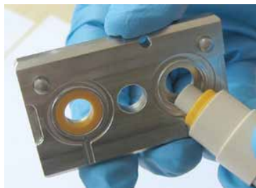
Fig. 55: Inserting the piston seal into the plate of the rear seal wash system
