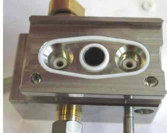
Fig. 48: Seal installed in the pump head
