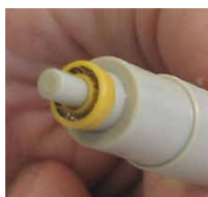
Fig. 47: Correct orientation of the piston seal (here reversed phase)
