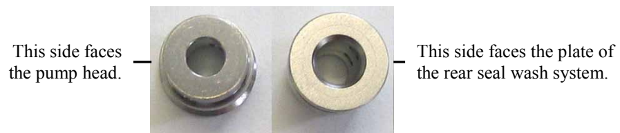
Fig. 49: Orientation of the rear seal wash body
