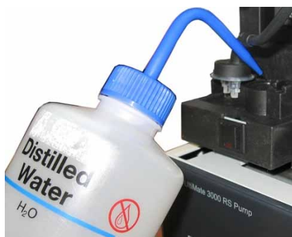
Fig. 19: Filling water into the connection port
